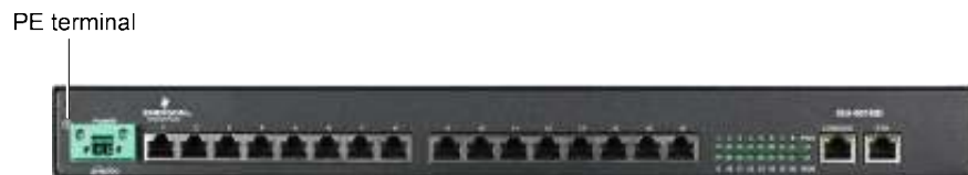
Figure 3-9 Position of PE terminal
