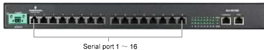
Figure 3-2 Position of ISU-0016ID serial port
