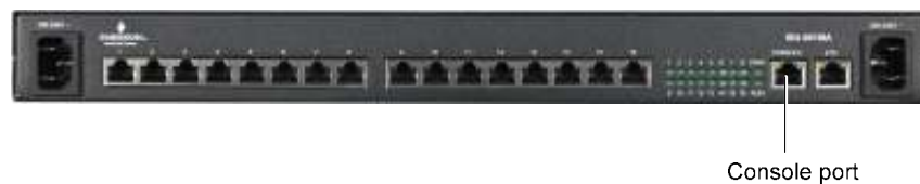
Figure 3-7 Position of console port
