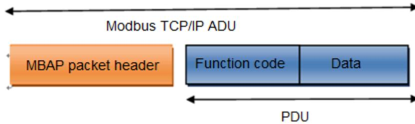
The MBAP packet header (MBAP is short for Modbus Application Protocol) is divided into four domains which include seven bytes in total.
