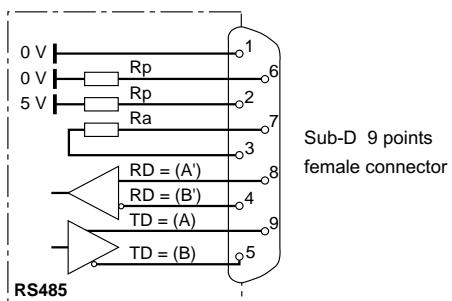
The default setting of the RS485 is a 4 wires configuration without polarity and without termination.
