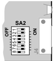
Link with polarity and without termination.
