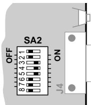
Link without polarity and with termination.
