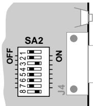
Link without polarity and with termination.
