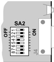
Link with polarity and with termination.
