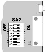
Link with polarity and with termination.
