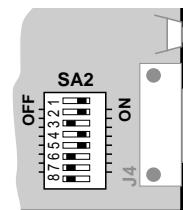
Link with polarity and without termination.
