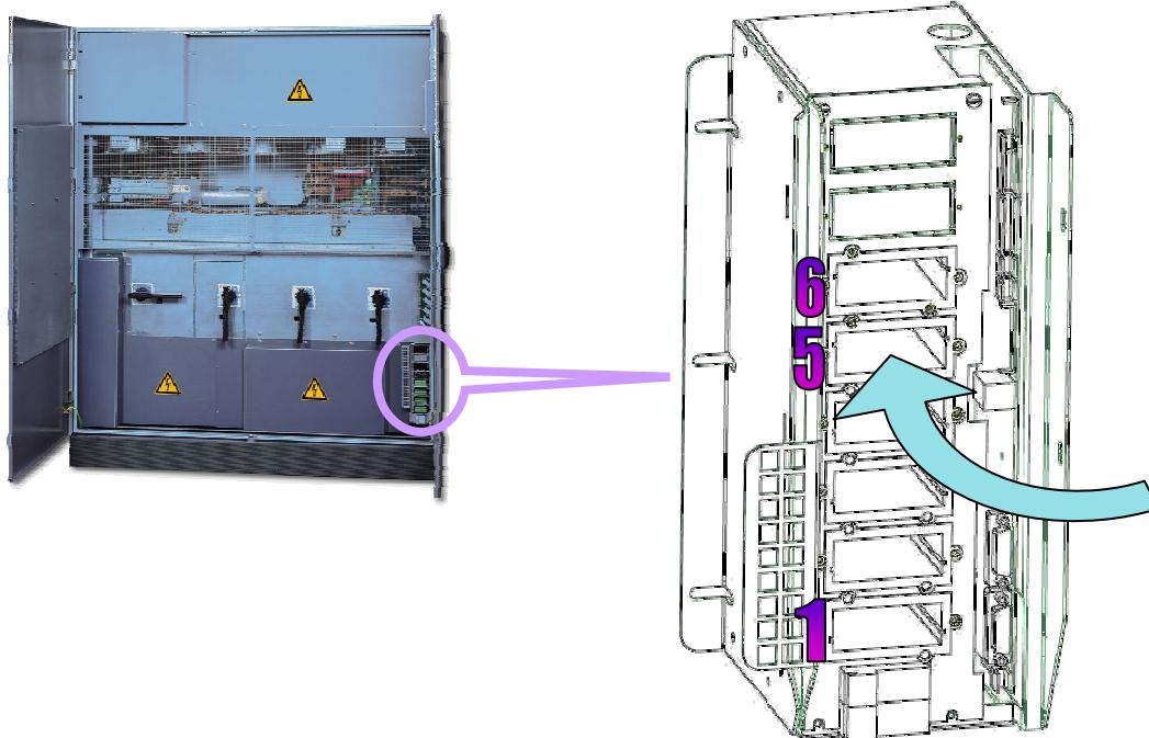
The « com-slots » includes all communication interfaces and is located in the lower right corner of the UPS.
